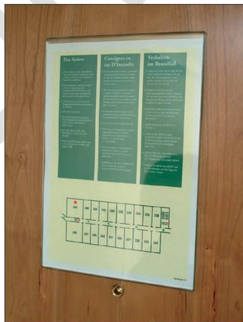
Figure 42: A typical bedroom fire procedure notice
