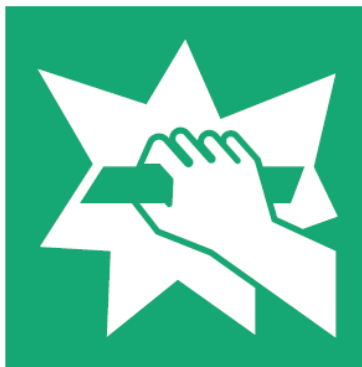
Figure 14: Suitable pictogram for emergency door release control (Other pictograms may be used, provided the meaning is clear)
